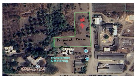
The proposed area for the location is as per the picture shown above. The Solar PV System proposed is a ground mounted Solar System under net metering. The system will be connected to the main bus bar at the LT room near the transformer.
