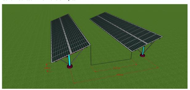
Ground Mounted Standard with Hot Dip Galvanized Columns, Rafters, Bracing, Hat Shaped Galvalume Purlin, SS 304 Fasteners for Structure and Module mounting. The design should be capable of withstanding wind speed of 160 kmph. The foundations should be of M25 concrete. The piling depth and the entire structural design should be certified by a Structural Engineer.
